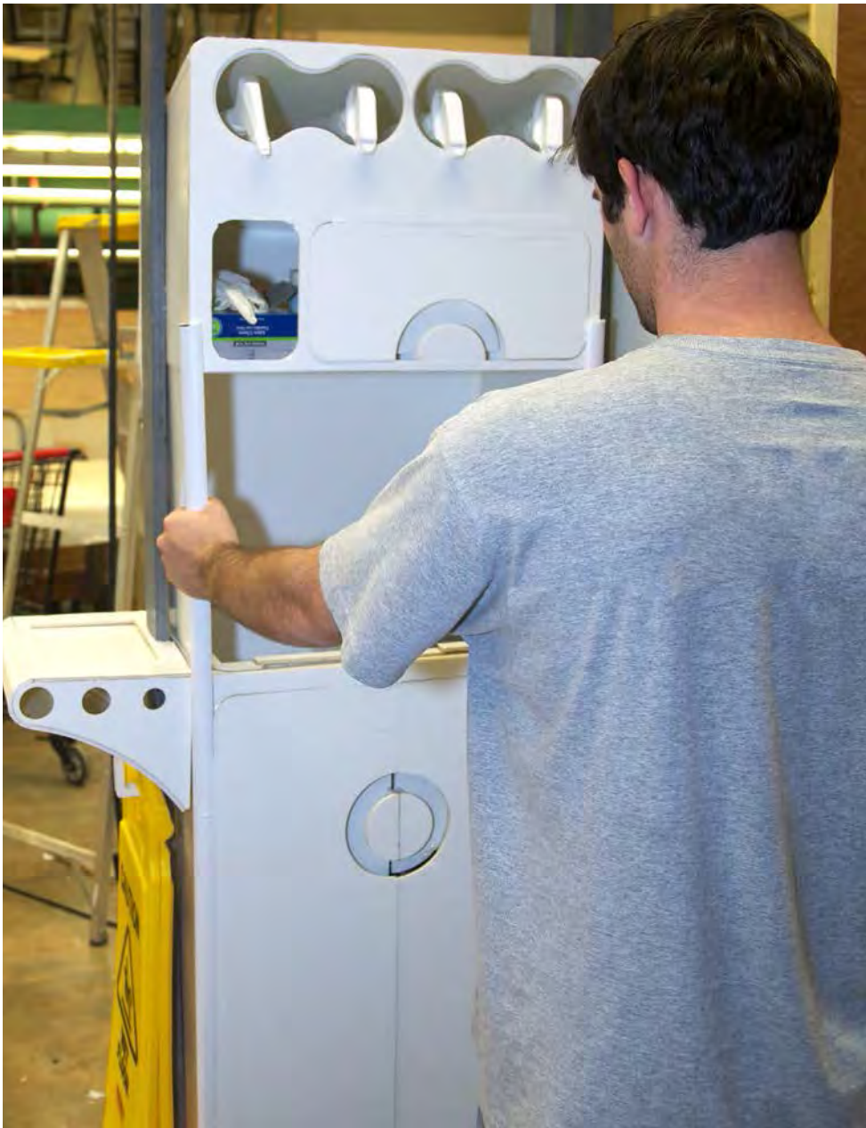
To make our product more user friendly we added a place for handles. This allowed the system to move from left to right inside the room.
