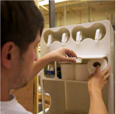
Placing the cleaning solution so high gave risk to spilling into eyes.
