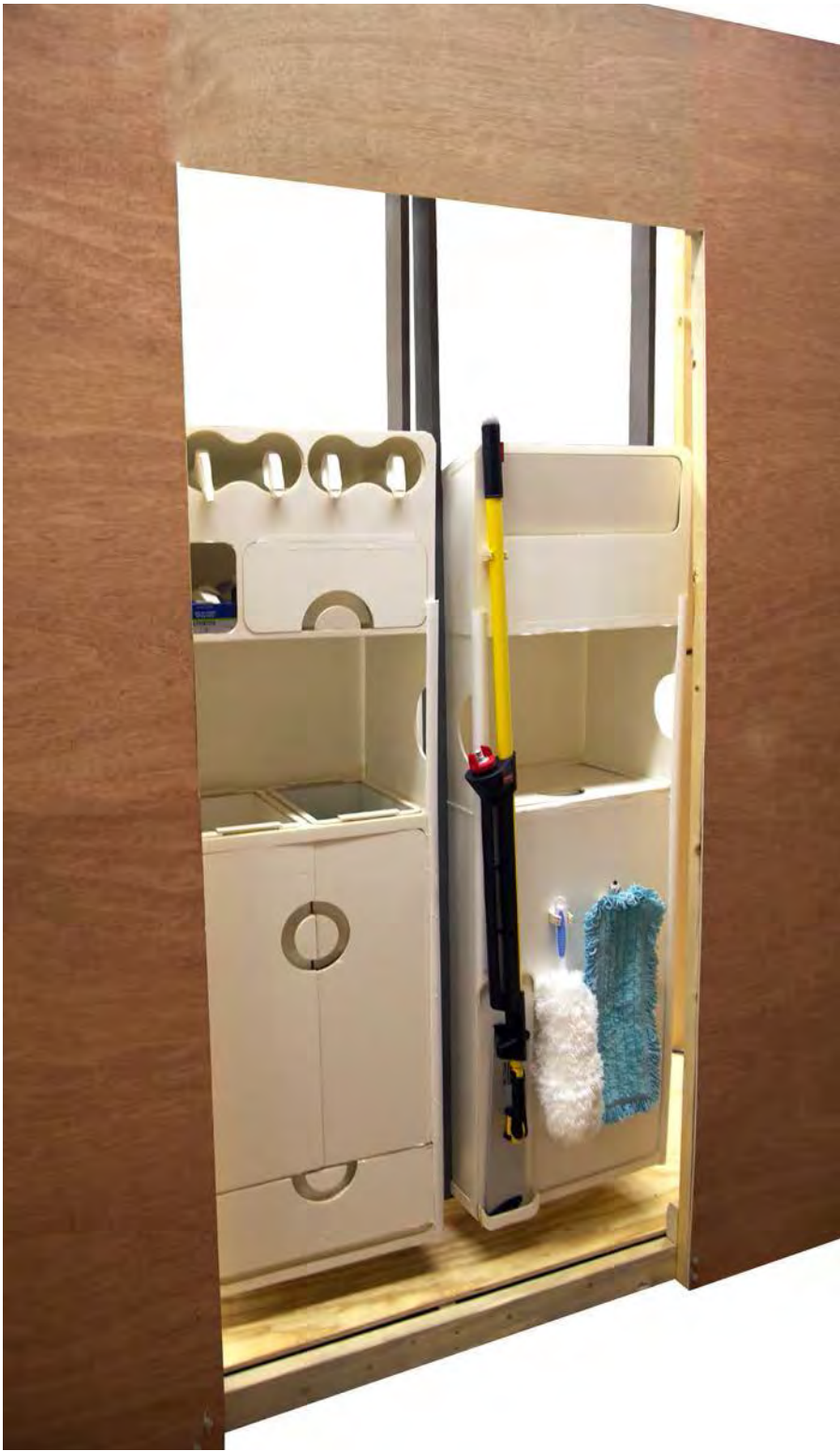
To make our product more user friendly we added a place for handles. This allowed the system to move from left to right inside the room.
