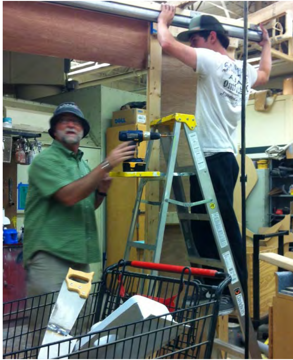
To simulate the rail system a barn door slider was installed to accurately mimic the movement of the system up and down a hallway.
